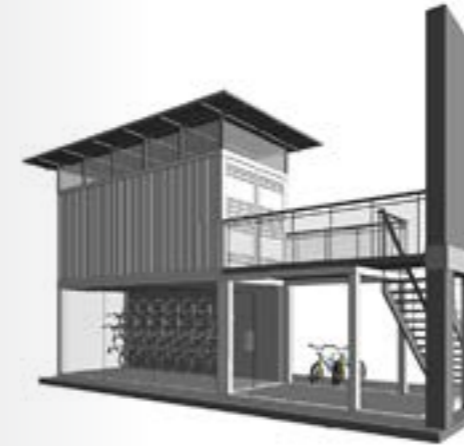
A double-storey version of the current bike station prototype: KLCSI is currently designing a prototype to be used as a pilot. This model has a simple design as a solution to a cost-effective approach. Solar panels are proposed to be fitted onto rooftop. Recycled cargo containers are also used as a sustainable practice.
